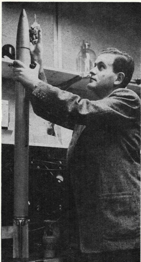
Dr. Fred Singer, MOUSE inventor, with a Rockair rocket and the tiny unit—consisting of a Geiger tube, a sound amplifier, a radio transmitter, and a power supply of 900 volts—which the physicist designed to fit into the 2\frac{3}{4} -inch diameter of the Rockair's nose cone.
